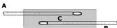
Figure 2. Zeroth law of thermodynamics: thermometers A and B do not exchange heat with system C, then A and B are in thermal equilibrium. If two systems are in thermal equilibrium, their temperatures are defined as equal, so A and B have the same temperature.
