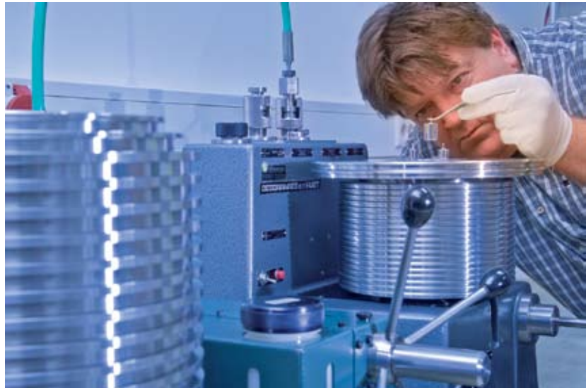
The skills of personnel is the dominant factor for the laboratory's performance. The assessor will want to look at training records and observe technicians at work. Here, Jos Verbeek of the Dutch Metrology Institute, adds a mass piece on a pressure balance.
