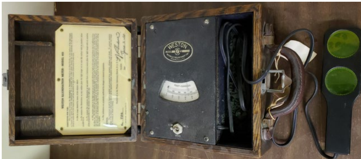
Weston Model 603 Light Meter with originally colored photocells, circa the 1930s.
