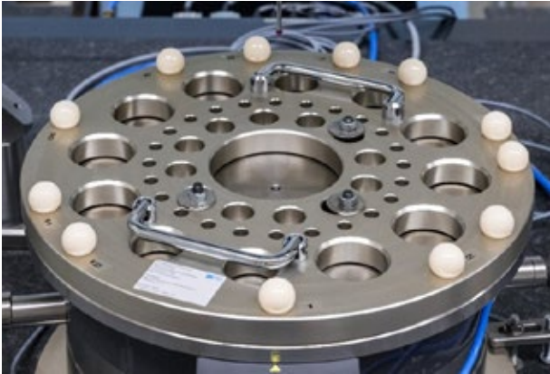
Ball plate for the reduced three-rosette method with 12 irregularly arranged balls. Credit: PTB
