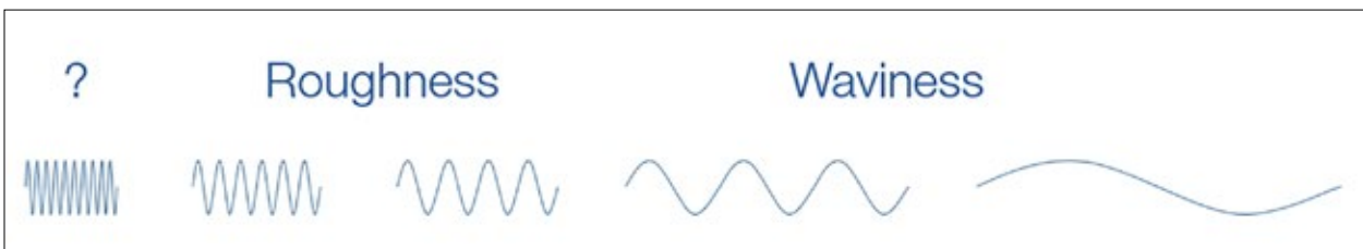
Figure 3. Surface texture consists of a spectrum of feature sizes and spacings.
