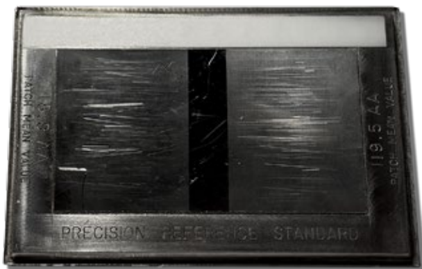
Figure 8. The location and direction of measurement on this calibration patch can produce vastly different R_a values.
