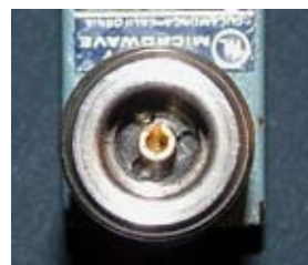
Figure 5. 7-mm connector with gouges.
