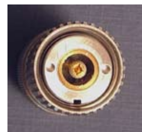
Figure 6. Type-N female connector with missing pin segment.
