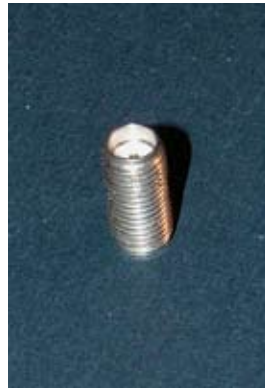
Figure 1. Threads Damaged by Pliers
