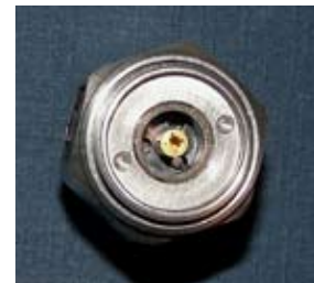
Figure 4. 7-mm connector with missing plating.
