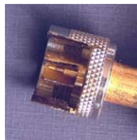
Figure 7. Type-N male connector with pin wear.
