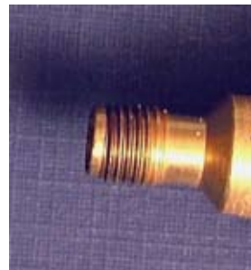
Figure 3. 3.5-mm female connector with missing plating.
