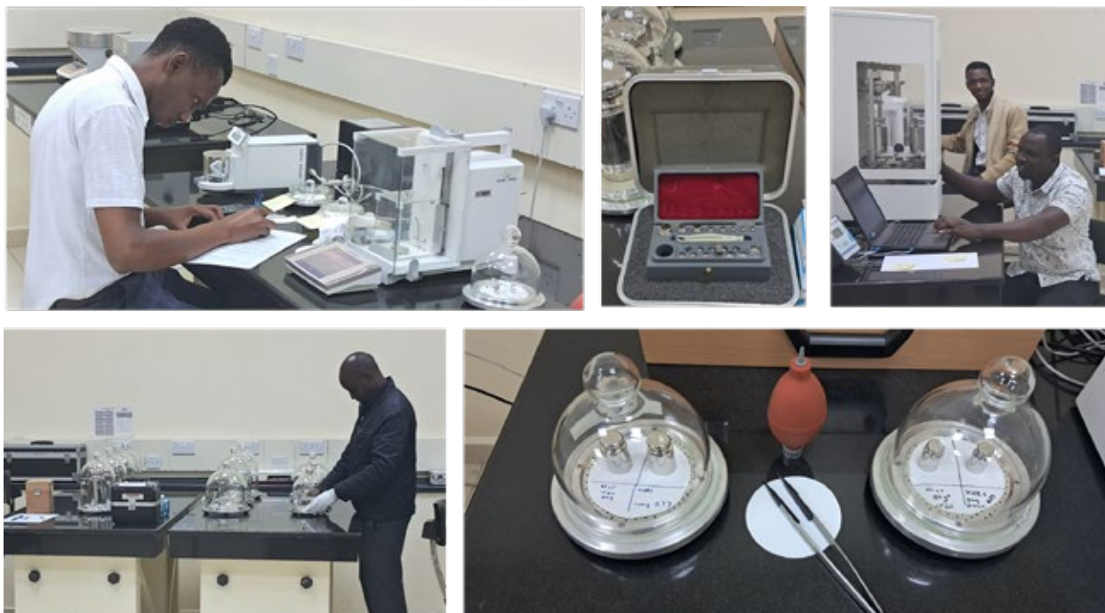
KEBS mass metrology staff measure the values of a NIST mass comparator set in a 2024-2025 NIST-KEBS bilateral comparison. The mass set will be transported back and forth between Kenya and the U.S. and its values compared at NIST and KEBS metrology laboratories over the course of a 1-year period. Credit: O. Nyangau/KEBS
