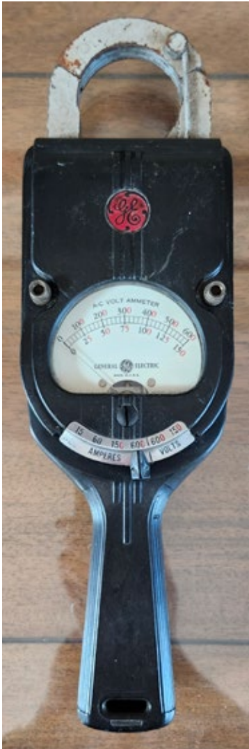
Picture 11 and 12. GE Clamp-on current meter and portable watt meter manufactured at the GE plant in Schenectady, NY.
