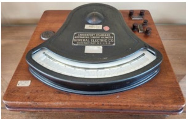
Picture 13, 14, and 15. Laboratory standards for the Alvin S. Mancib Company, replaced by calibrators in the late 1970s.
