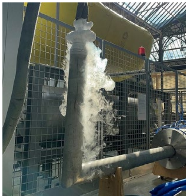
The cryogenic flow rate test rig provided by the Karlsruhe Institute of Technology (KIT) when operating with liquid nitrogen at PTB. Credit: PTB
