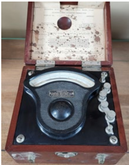
Picture 2. GE Type P3 Ammeter calibrated May 20, 1911.
