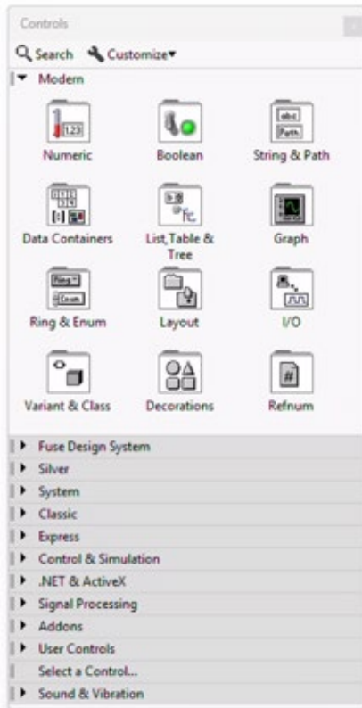
Figure 3. Control palette with various controls (inputs) and indicators (outputs) that goes into the front panel.
