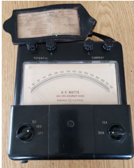
Picture 11 and 12. GE Clamp-on current meter and portable watt meter manufactured at the GE plant in Schenectady, NY.
