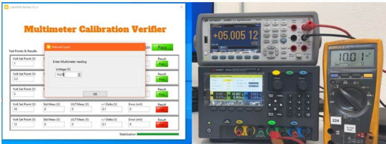
Figure 8. The screenshot demonstrates the execution of a calibration verifier tool, which automates the setting of power supply values and reading of high-precision DMM measurements, while allowing manual entry of values from a hand-held DMM.
